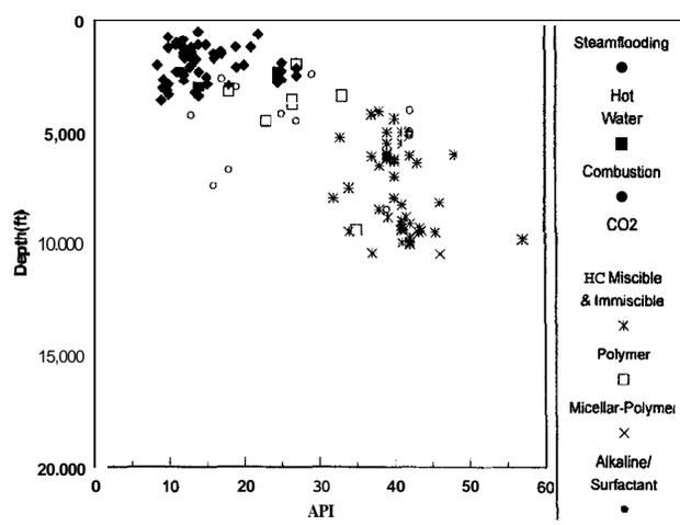
**Fig. 4—Depth and oil gravity of producing EOR projects outside the U.S. (data from Ref. 25).**
