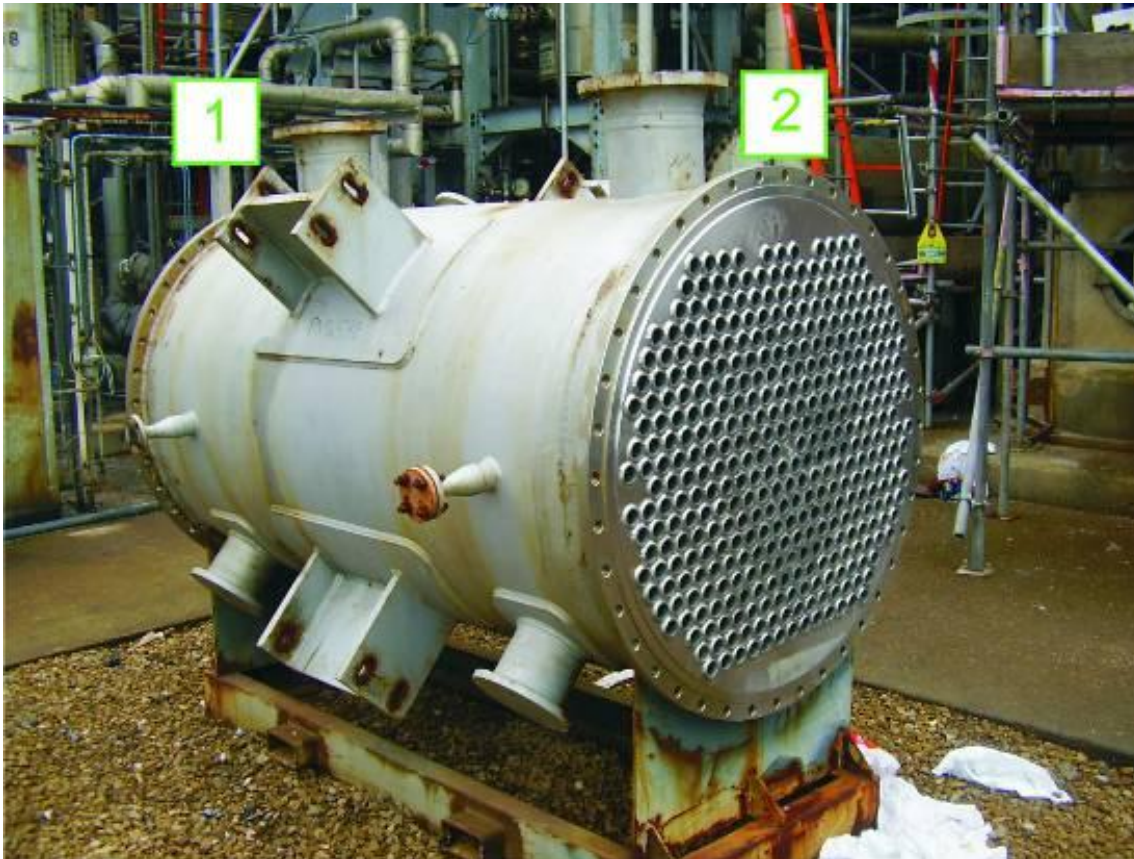
Figure 4 A tubular reactor used in the production of methyl 2-methylpropenoate . The reactor is heated by high pressure steam which has a temperature of 470 K and is fed into the reactor at point 1 and leaves the reactor at point 2. The reactants flow through the tubes.
